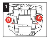
Move seat to fully reclined position. Push down on tab on right side of base (A).
